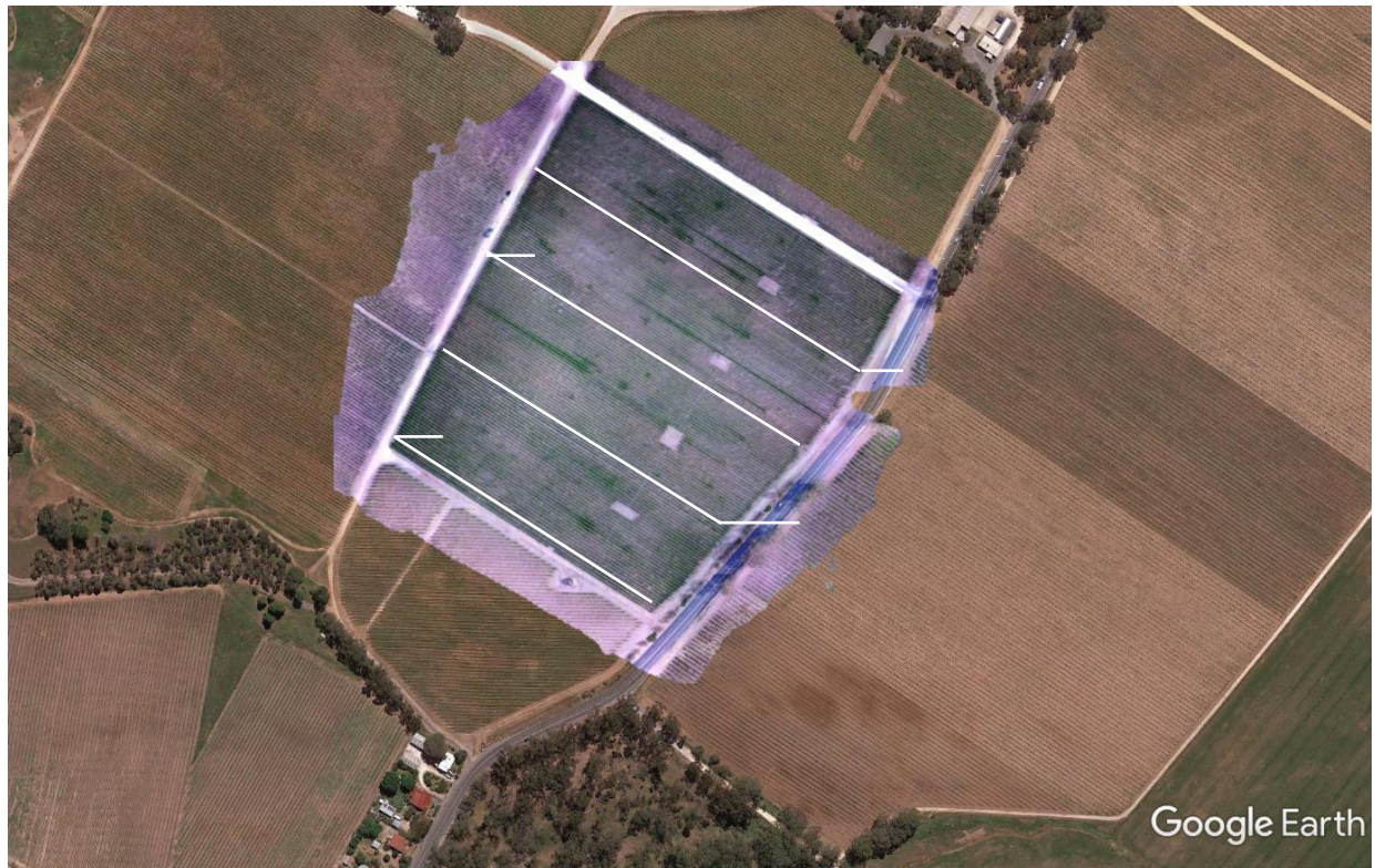
Figure 7: Orthomosaic view of the VIS dense point cloud superimposed onto a Google Earth extract of the Jacobs Creek site at 34° 34' 04" South, 138° 56' 00" East. The white lines depict the approximate 'lawn mower' flight.
