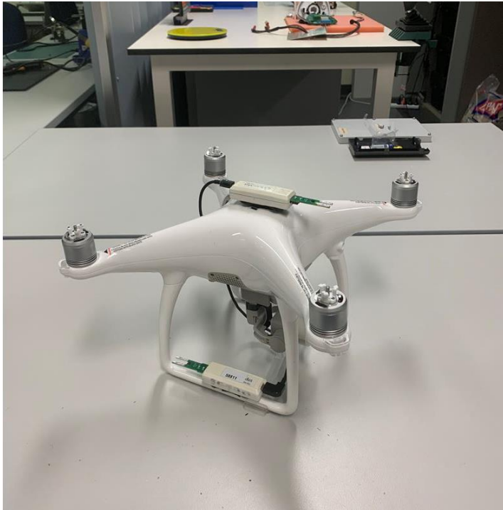
Figure 10: Meteorological sensors mounted above and below a Phantom IV UAV. They are placed above and within the airstream generated by the UAV's propellers to capture meteorological measurements. The meteorological sensors can measure pressure ( \pm 1.5\text{hPa} ), temperature ( \pm 0.3^\circ\text{C} ), relative humidity ( \pm 5\% ), and location ( \pm 5\text{m} ) simultaneously at a rate of 1Hz (note: the UAV's propeller blades are removed as a safety precaution while it is in the laboratory).
