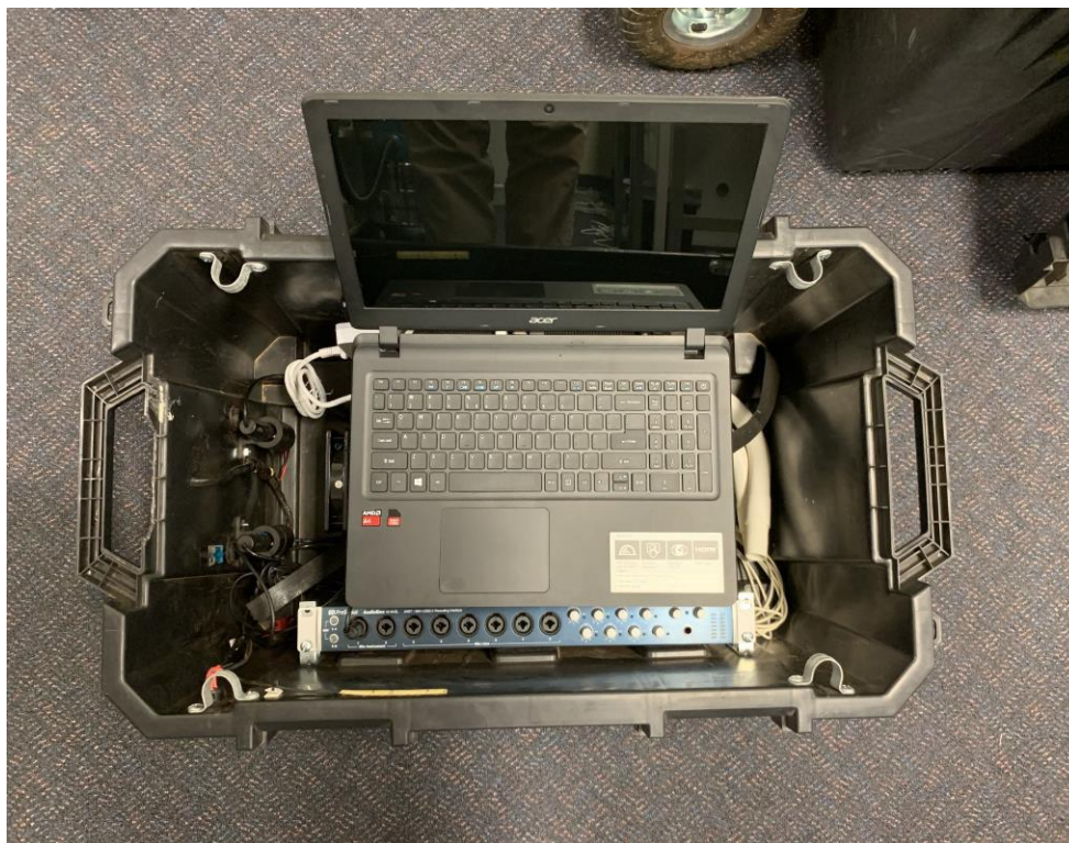
Figure 9: Ground station (one of seven), comprising a laptop that manages and records data from an 8-channel, 24-bit DAQ with 107dB spurious free dynamic range. 7 channels sample ECM800 10mV/Pa condenser microphones at 44.1kHz. Accurate time timing is maintained by sampling the GPS-derived 1PPS edge on the 8 th channel.
